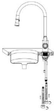
Install the flexible hoses with inlets in the body. These should be hand tightened, do not use a spanner as this can damage the O – ring.
