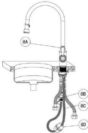
From underneath the sink, fix the lead(8D) with pull-out hose(8C), and tighten the screws on the lead after the hose is properly adjusted for suitable length.
