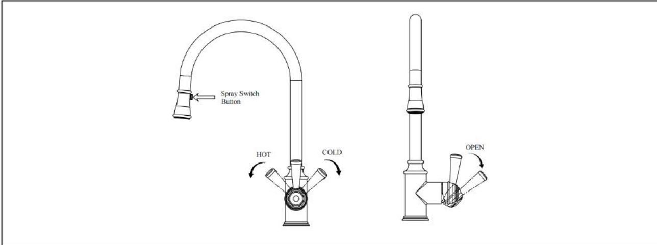
The pull-out hand sprayer has 2 functions. Standard mode is AERATED FLOW. By pressing the switch button, the mode becomes SPRAY. The mode automatically gets back to standard when the mixer is closed and re-opened.
