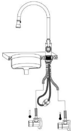
Connect the hot and cold flexible hoses to the isolation valves (not included), hot on the left, cold on the right.
